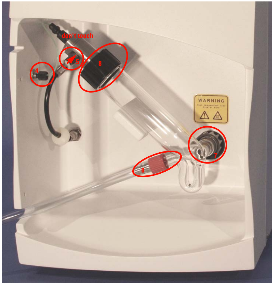
Figure 17 Replacing the nebulization chamber
