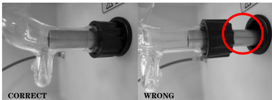
Figure 12 Fixing the Tip of Nebulization chamber
